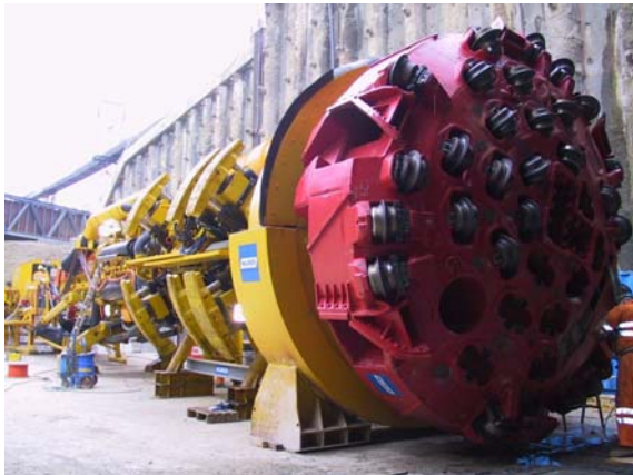
Pilot TBM being assembled
