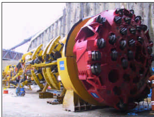
Cutting head of Pilot TBM (5m diameter)
